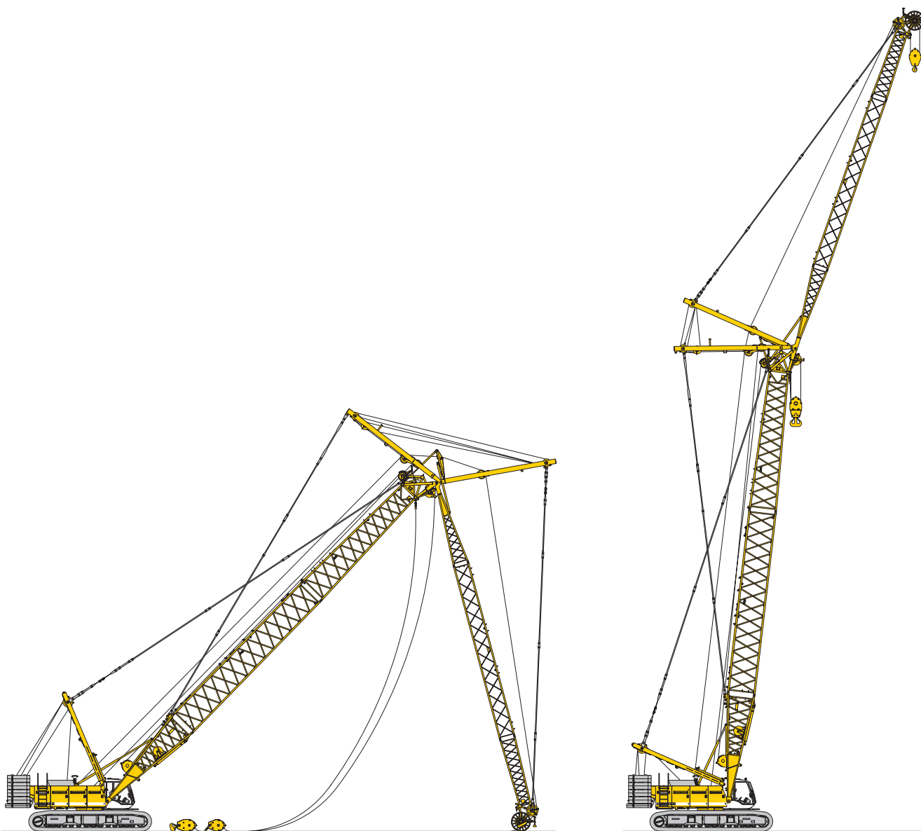
Erecting of main boom and luffing jib
