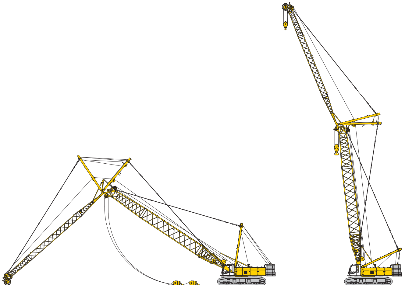
Erecting of main boom and luffing jib
